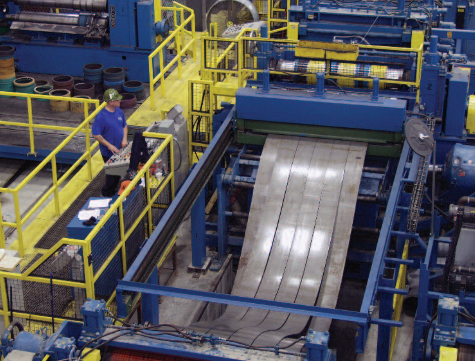
Mississippi Steel Processing's 0.25-inch by 72-inch Pro-Eco slitter in operation.
